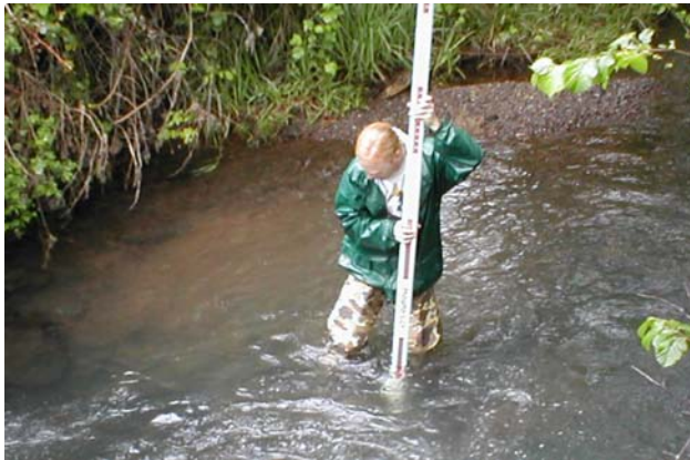
Photo 4. Culvert 323 in the headwaters of Brush Creek. Below the culvert outlet collecting maximum scour pool depth measurements.
