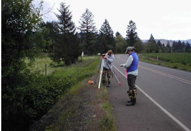
Photo 3. Culvert 435B where Brush Creek Road crosses West Fork Brush Creek. Setting up the transit for the field survey and recording location information with the GPS.
